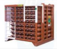
64 cylinder Quad DNV 2.7-1 Dimensions (L x W x H): 1.8 x 2.1 x 2.3 Weight (filled with nitrogen at 300 bar): 6,400 kg Volume (filled with nitrogen at 300 bar): 831 m3
